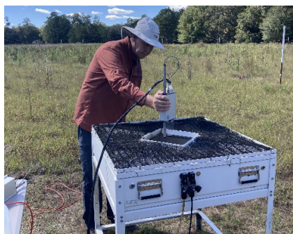
MonoJet-LDG being used to field calibrate a Joanneum 2DVD disdrometer at College of Charleston (SC)
