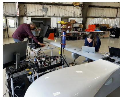
MonoJet-CMAG being used to validate calibration of an aerosol probe deployed on the DOE ARM ArcticShark UAS
